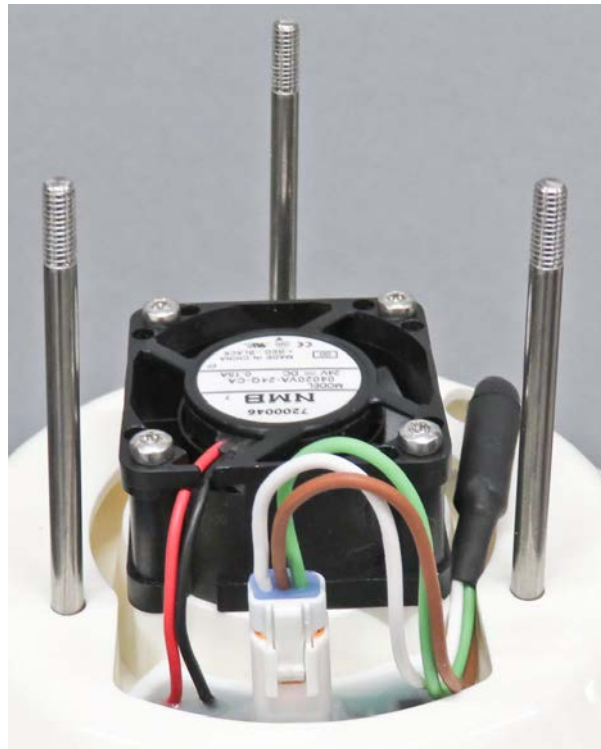
Figure 5: Cable routing after replacing the fan assembly
