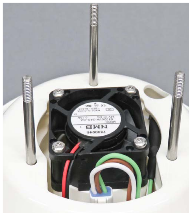
Figure 6: Cable routing after putting on the second protective cap
