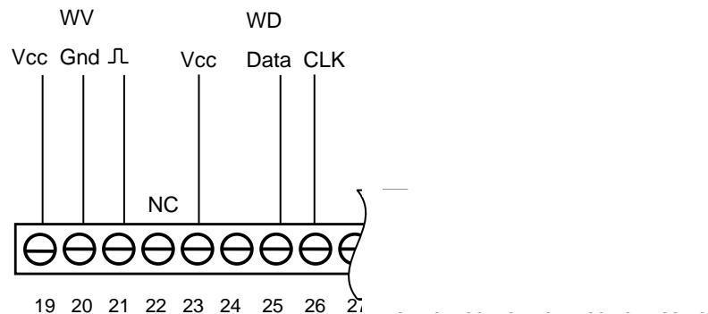
**Figure 10: Connection of digital combi wind transmitter**
