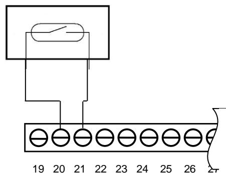
**Figure 11: Connection of wind transmitter with reed contact**
