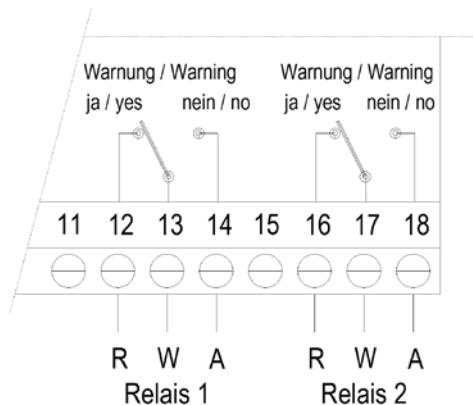
Figure 12: Relay output
