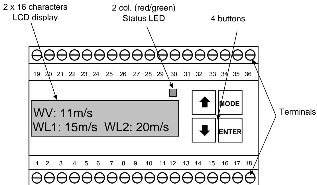
Depending on the wind alarm type selected, four main menus with the following menu items are available for operation and programming of the wind alarm unit.
