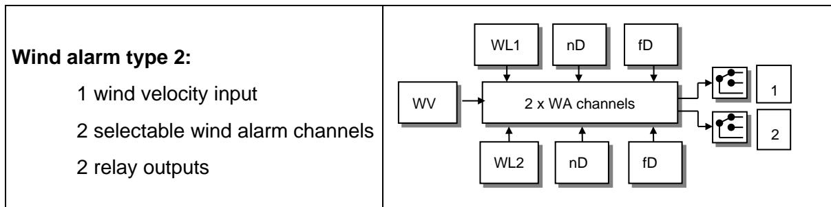
Figure 5: Wind alarm type 2
