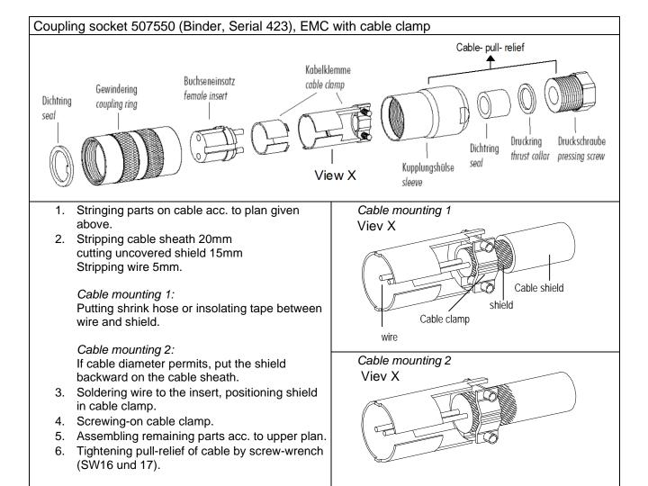
Figure 1: Coupling socket installation
