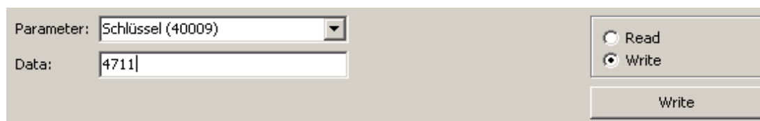
Figure 11: Terminal for MODBUS-RTU interpreter (write)
