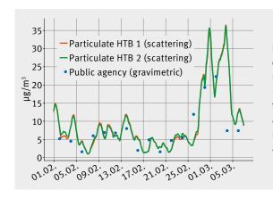
PM2.5 measurement results of two Thies CLIMA particulate matter measuring devices (Particulate matter-hygrothermo-baro sensor compact) and a close-by gravimetric measurement of a public agency.
