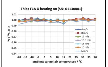
Five anemometers have been tested. Each individual temperature-ratio data have been used for classification
