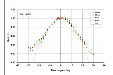
Five anemometers have been tested. Each individual tilt data have been used for classification
