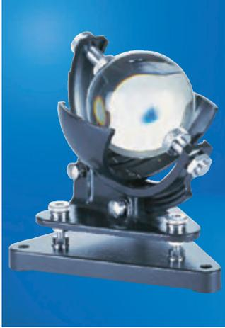
Registers the sunshine duration for one entire day. A cut glass sphere focuses the sun's rays and leave an image line on the strip chart. The length of the image line corresponds to the duration of sunshine. The shipment includes the following strip charts
