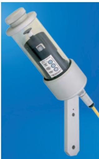
Instrument to measure the sunshine duration and direct radiation.
