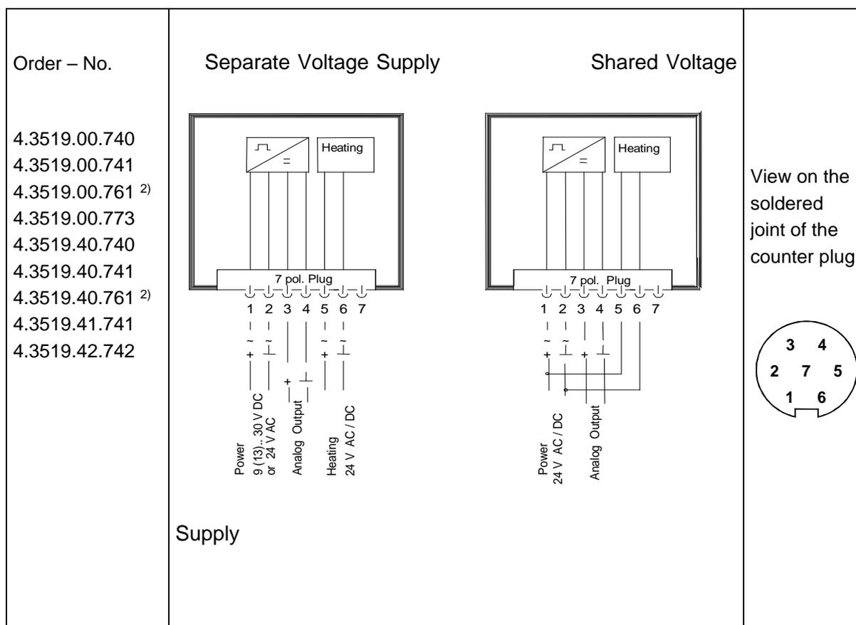
**Figure 3: Connecting Diagram for Models with Connector**
