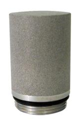
Sinter Filter ZE 21 1.1005.54.902 This basket is placed over the sensor and protects the measurement element from high wind speed (5 m/s) and increased dust. A necessity for sensors in use in exposed areas, eg. in marine climates, desert, mountains.
