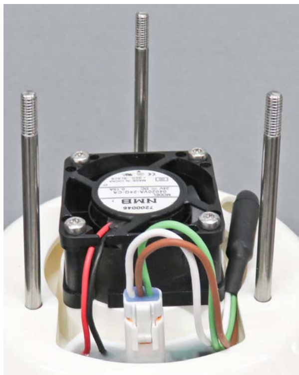
Figure 5: Cable routing after replacing the fan assembly
