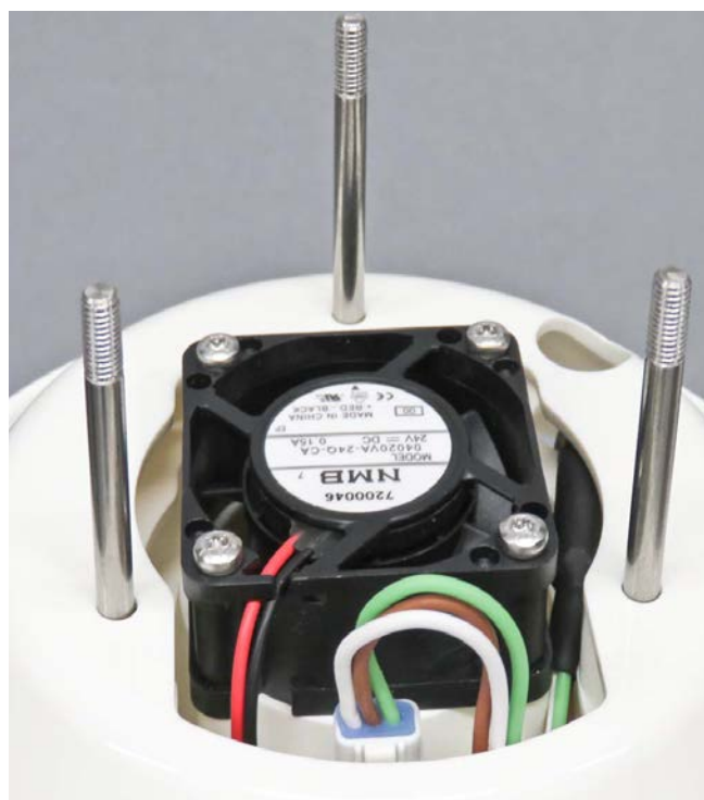
Figure 6: Cable routing after putting on the second protective cap
