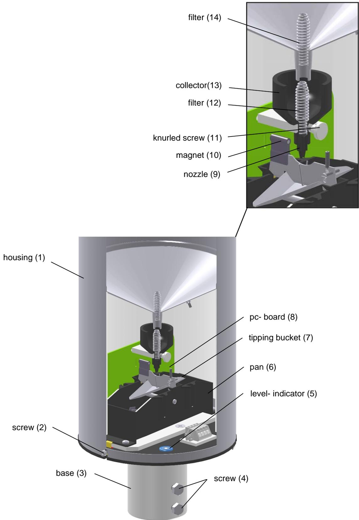
**Figure 1: Instrument construction**
