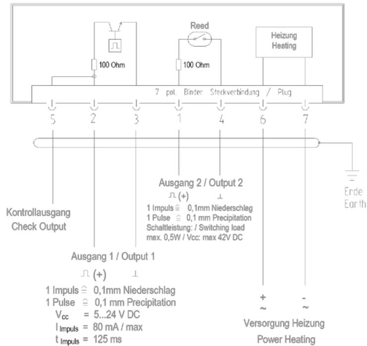
View on the soldered joint of the counter plug.
