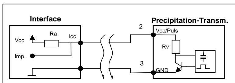
Figure 3: Example - Connection to a Interface
