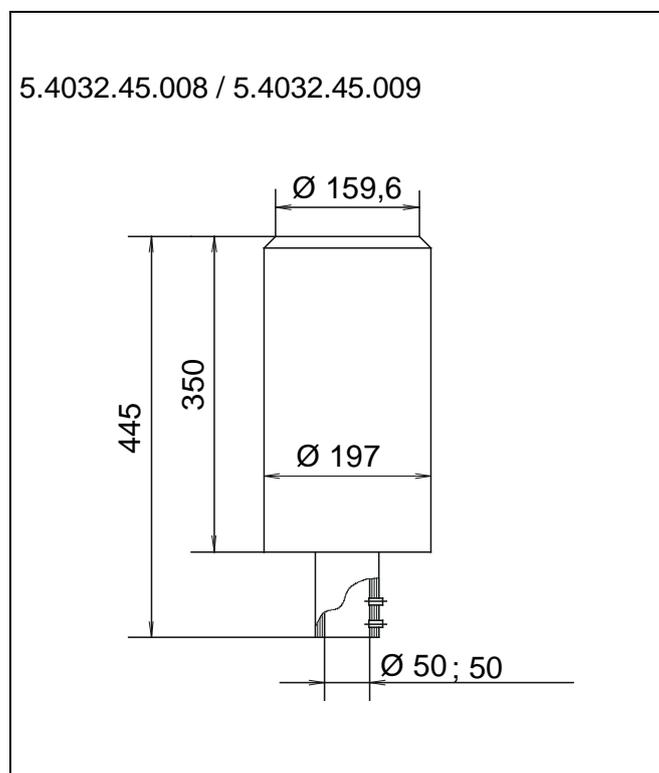
**Figure 6: Dim. drawing Precipitation transmitter with casing heating**
