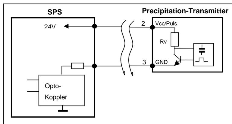
Figure 4: Example - Connection to a SPS
